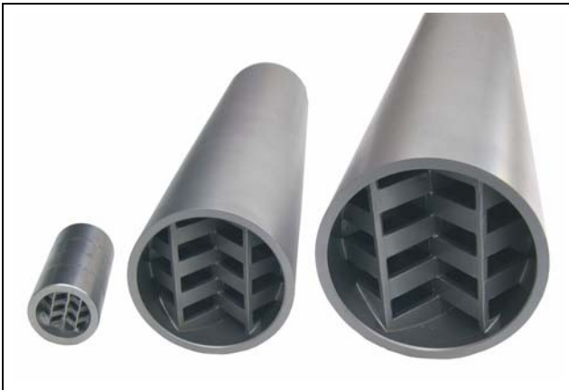
Figure #4: SMB-S Sleeve Type Mixing Elements where the 8-SMB-R Mixing Elements are welded together into a single assembly. Used for special applications where single-piece construction is required such as in deep bore one-direction access applications.
