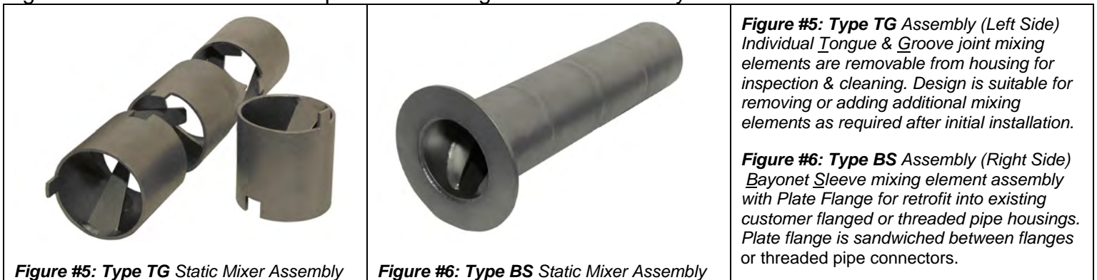
Figure #5 & #6: Construction Options for Mixing Element Assembly
