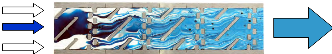
Mixing Pattern of High Performance Type GXR Static Mixer (Not Medium Performance Type VF Static Mixer described in this brochure)
