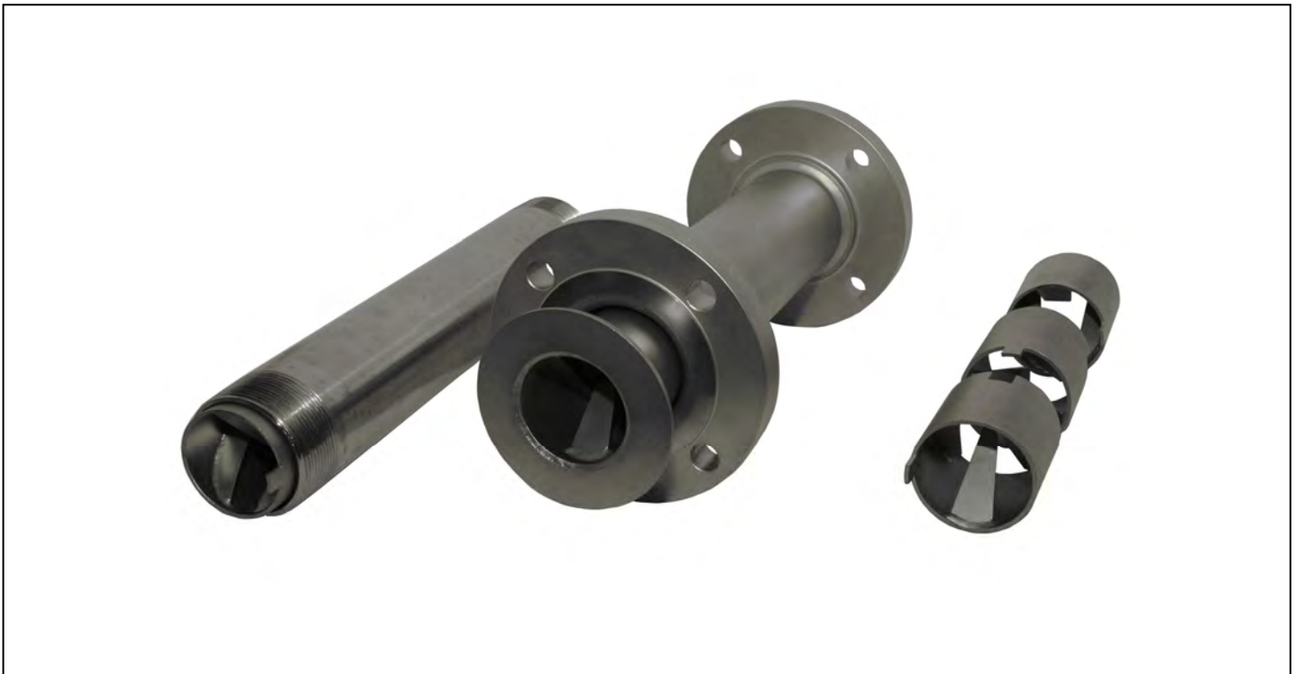
Figure #1: The StaMixCo Sludge Blender contains Type VF Static Mixing elements that can be removed from the housing for inspection and cleaning (right side photo). The mixing elements may be mounted in a pipe with threaded end connections (left side photo) or a pipe with flanged end connections (center of photo). For existing installations with flange connections, the Type VF static mixer is available as a Model BS sleeved unit with a plate flange (center photo) that slips into existing piping and is supported by the plate flange which sandwiches between the raised face of adjacent flanges in the piping system.
