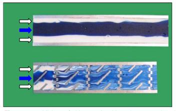
**Figure #5:** Mixing of blue and white viscous resins is demonstrated (1:1 volumetric ratio). In an empty pipe (top), no mixing occurs. With eight SMB-R mixing elements, a high degree of mixing is achieved in a short length.
