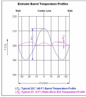
**Figure #2**: An extruder screw (blue line) typically delivers molten polymer with a high temperature gradient which effects product quality. The Type SMB-R and SMB-GX mixing elements reduce the temperature variation to less than 3  $F^{\circ}$  (purple line).
