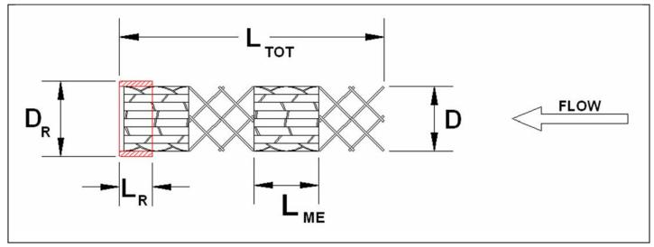
Figure #18: Dimensions of four (4) SMB-GX mixing elements (see Table #2)
