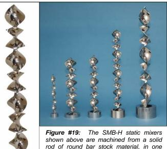
shown above are machined from a solid rod of round bar stock material, in one piece and without welding. The machining process allows any L/D twist to be supplied. The second static mixer from left is L/D=0.7; the fourth static mixer from left is L/D = 1; and the remainder are L/D = 1.5.
