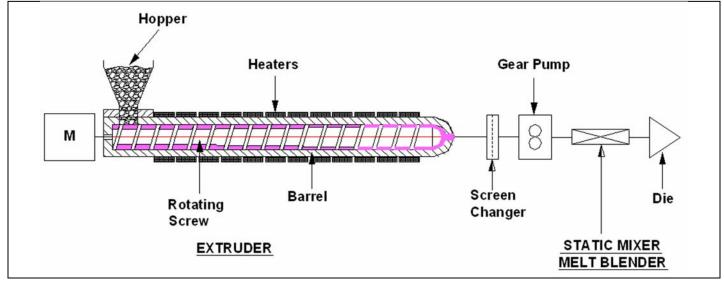
Figure #1: The Static Mixer Melt Blender is installed just in front of the die to homogenize the polymer melt.
