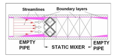
**Figure #8:** A static mixer retards the formation of a boundary layers along its entire length. In addition, it homogenizes into the bulk stream all irregularities created by upstream equipment such as extruder screw & piping boundary layers and colorant hang-up release, gear pump teeth footprints and flaking off of wall-creep degraded polymer hang-up.
