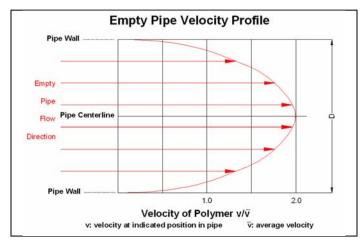
Figure #6: Velocity profile in an empty pipe.
