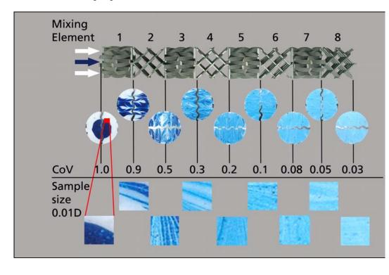
**Figure #17**: Blue and white viscous resin (1:1 volumetric ratio) is pumped through eight (8) SMB-GX static mixing elements, allowed to harden and cross-sectional cuts are made at the outlet of each mixing element.
