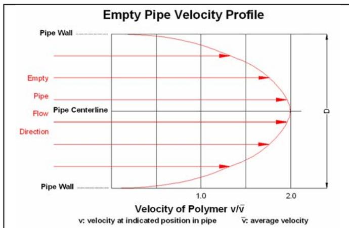
**Figure #6:** Velocity profile in an empty pipe.
