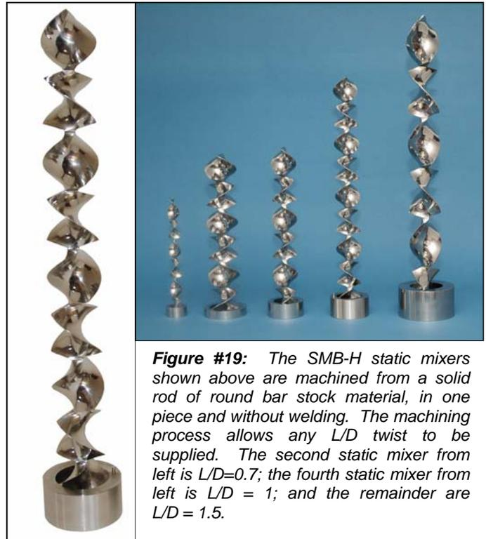
**Figure #19:** The SMB-H static mixers shown above are machined from a solid rod of round bar stock material, in one piece and without welding. The machining process allows any L/D twist to be supplied. The second static mixer from left is  $L/D=0.7$ ; the fourth static mixer from left is  $L/D = 1$ ; and the remainder are  $L/D = 1.5$ .
