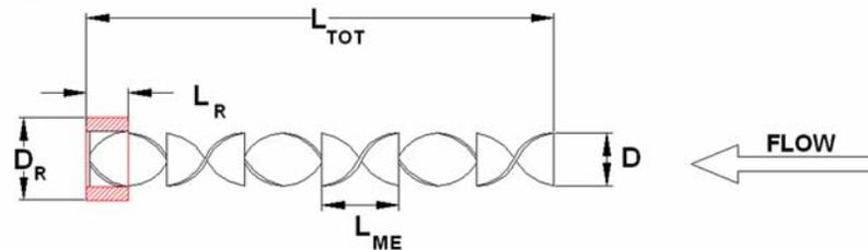
**Table #3:** Key dimensions of SMB-H Helical Melt Blender with 6-Mixing Elements of  $L/D=1.5$  twist.
