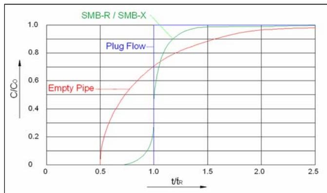
**Figure #9:** Step Response curve of Type SMB-R & SMB-GX mixing elements show good self cleaning abilities as compared to an empty pipe.
