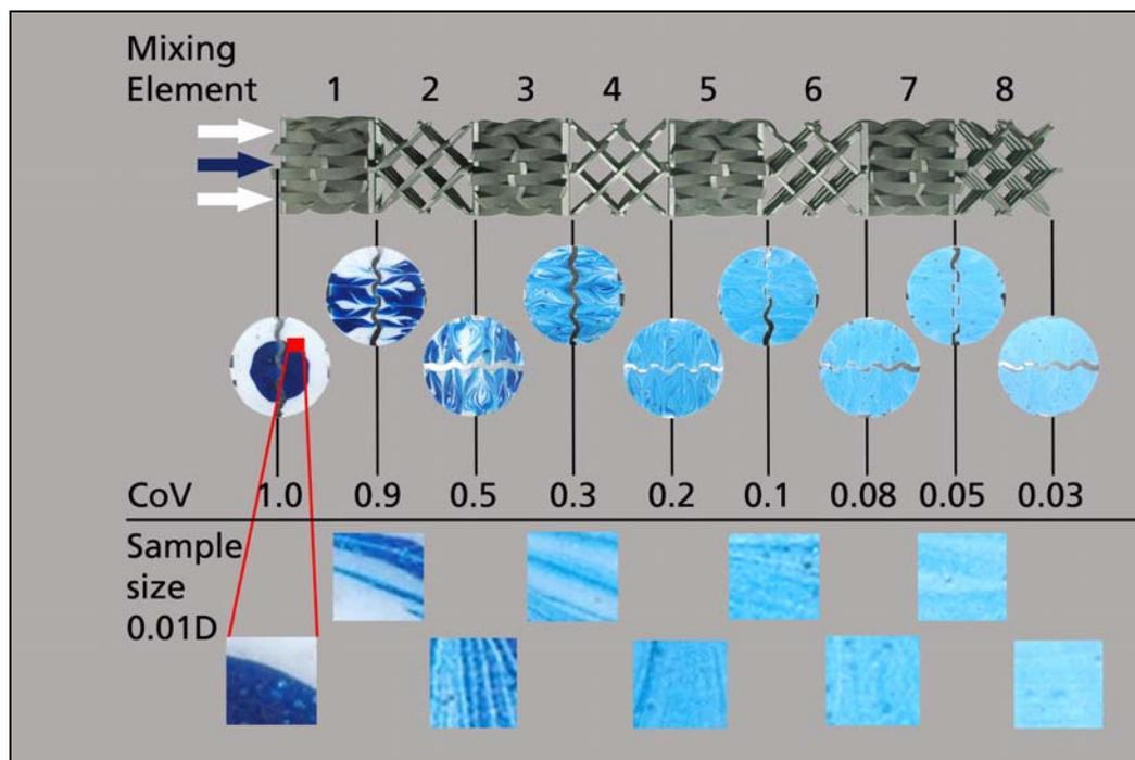
**Figure #17:** Blue and white viscous resin (1:1 volumetric ratio) is pumped through eight (8) SMB-GX static mixing elements, allowed to harden and cross-sectional cuts are made at the outlet of each mixing element.
