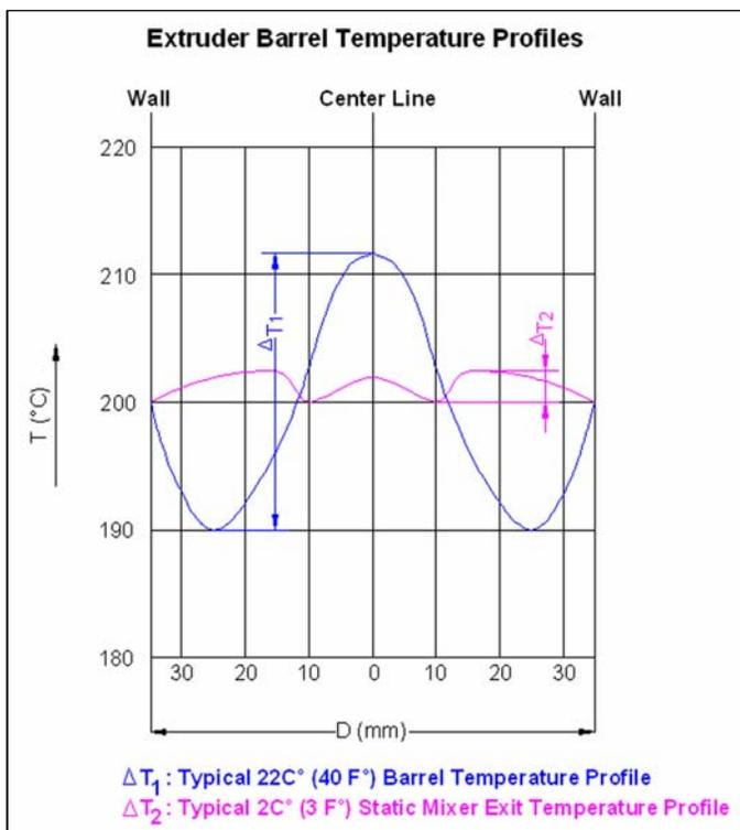
**Figure #2:** An extruder screw (blue line) typically delivers molten polymer with a high temperature gradient which effects product quality. The Type SMB-R and SMB-GX mixing elements reduce the temperature variation to less than 3 F°(purple line).
