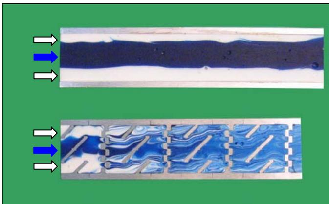
**Figure #5:** Mixing of blue and white viscous resins is demonstrated (1:1 volumetric ratio). In an empty pipe (top), no mixing occurs. With eight SMB-R mixing elements, a high degree of mixing is achieved in a short length.
